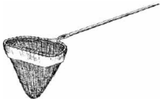
Figure 5-4. D-frame net used for collecting benthic macroinvertebrates.
