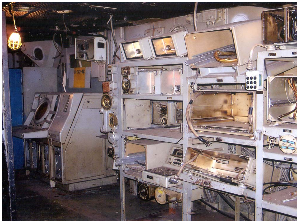
Photo courtesy of Laura S. Johnson Ex-USS Oriskany electronic equipment stripped of capacitors and transformers.
