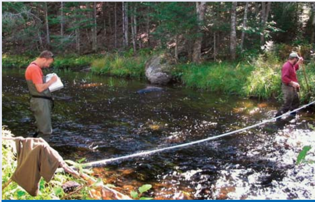
Habitat assessment data may include measurements of streamside vegetation and stream width, depth, and substrate (Photo courtesy of Colin Hill, Tetra Tech, Inc.).
