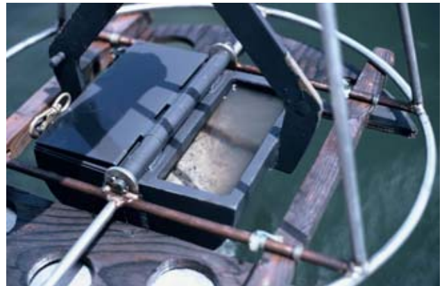
Ted-Young VanVeen sampler in supporting frame. Illustrating movable cover flap to enable direct sampling from the grab sampler. Note the overlying water in the sampler and adequate volume, indicating an acceptable grab sample.
