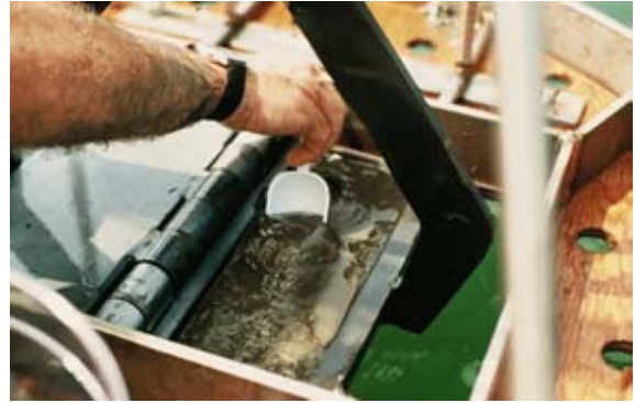
Taking subsamples from a Ted Young modified VanVeen sampler
