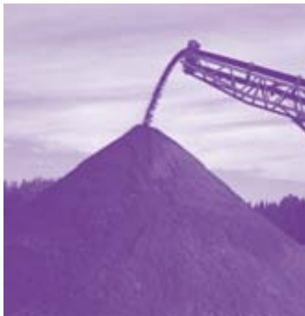
Crushed asphalt on conveyer belt.
