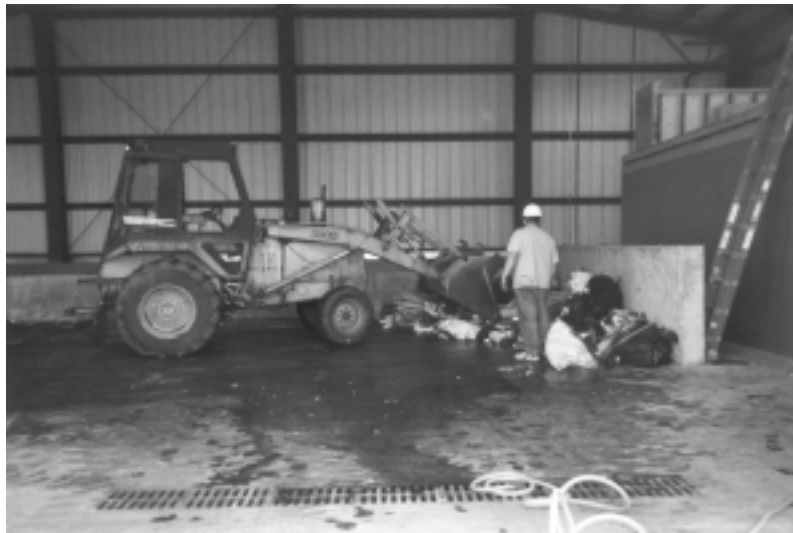
Front-end loader moving waste at the Eastern Band of Cherokee Indians' transfer station.
