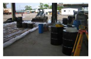
The HW storage area is located across the road (west) from the gasoline bulking area. Drums are stored here until they are categorized. After Hazcat testing, they are transferred to the drum storage/shipping pad for shipping. The observer should watch for leaking drums and tears in the liners. Drums placed here should have a tracking ("T") number marked on them; START also marks these drums with a "D" number for tracking purposes.
