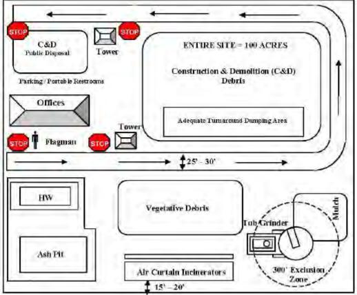
Figure 2. Example of a Debris Management Site
