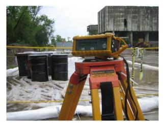
The air monitors measure LEL (Lower Explosive Limit),  $O_2$ , CO,  $H_2S$ , and VOCs. The monitor at the Special Refrigerator Storage Area monitors  $SO_2$  in place of CO. The monitors in the Oxidizer Section and the Hazcat Section also monitor for  $CL_2$  in place of  $H_2S$ . The monitors in the Oxidizer Section, Hazcat Section, Gas Tank Bulking Area/HW Hazcat Area and Special Refrigerator Storage Area also have Gas Alert single gas monitors for Ammonia.
