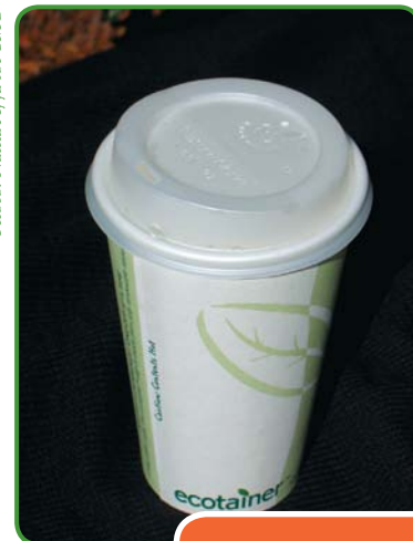
Moscone vendor SAVOR-Catering conducted rigorous testing before using NatureWorks's newest coffee cup lids made from PLA. Compostable coffee lids must be resistant to expanding from the effects of coffee's steam.
