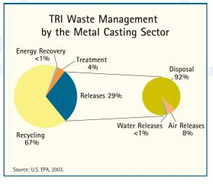
casters, accounted for the remaining 6%. Metals accounted for most of the quantity of TRI chemicals disposed or released by the sector. For example, manganese and zinc accounted for 63% by weight of total releases and disposal; chromium, lead, and copper accounted for another 23%.
