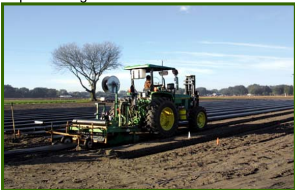
Raised Bed Shank Fumigation on wheeled tractor mounted shanks a depth of 8-12" and plastic tarps covering only the treated plant beds only.
