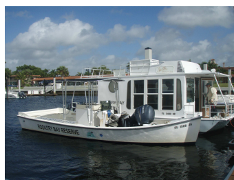
Rookery Bay NERR's mullet boat with its motor cleverly located in a forward well. This arrangement makes fouling the prop in nets unlikely and is also convenient for RBNERR's monthly shark long-line and gill net surveys.
