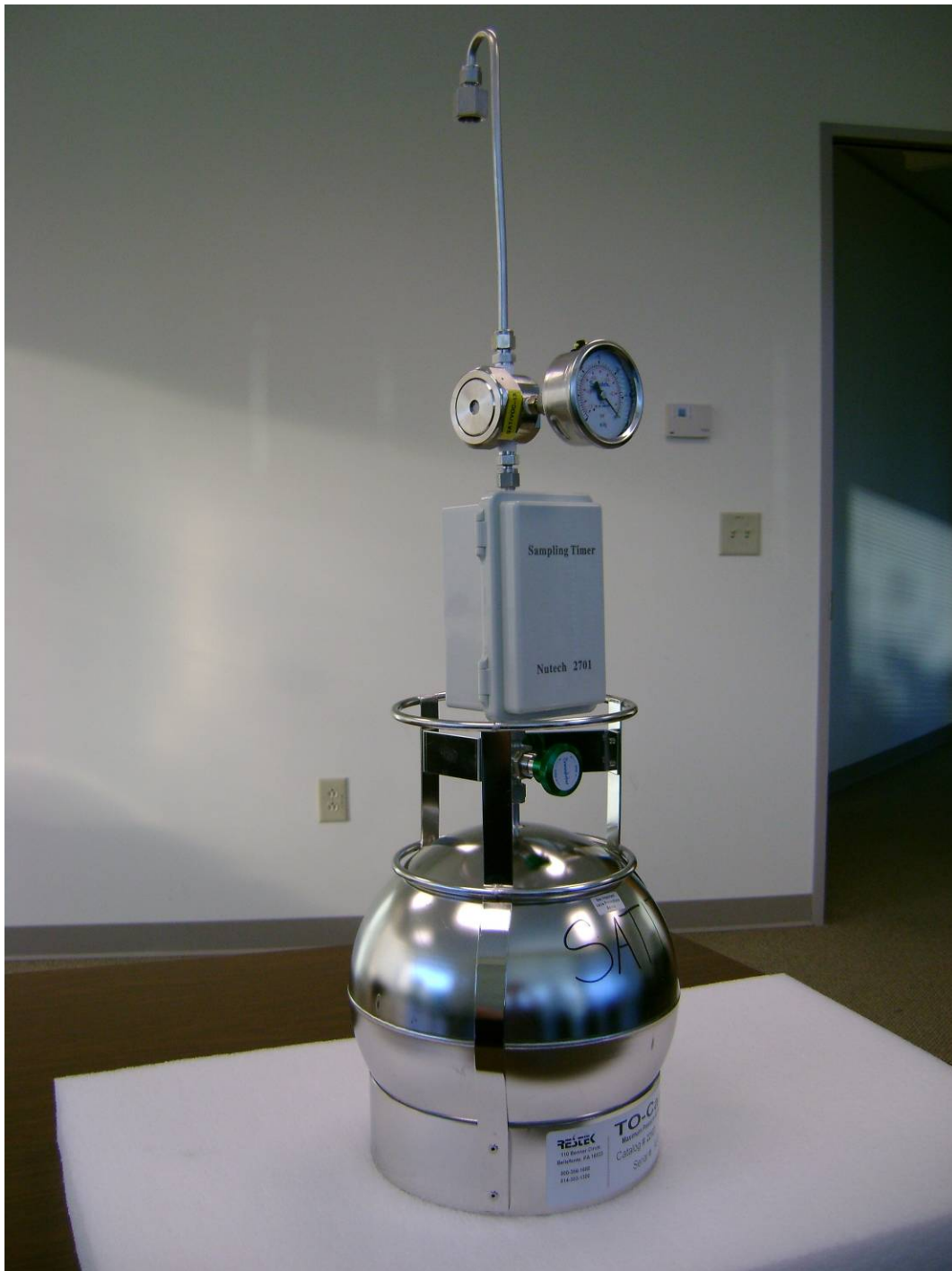
FIGURE 1. Photograph of Total VOC Sampling System With Timer and Probe
