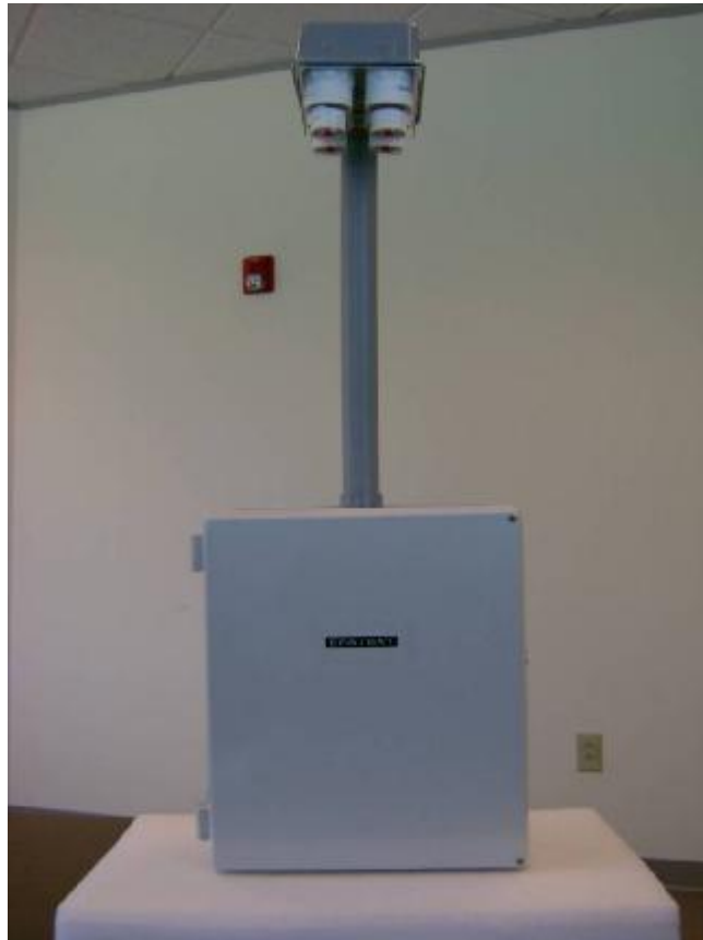
FIGURE 2. Diisocyanate Sampling System Enclosure
