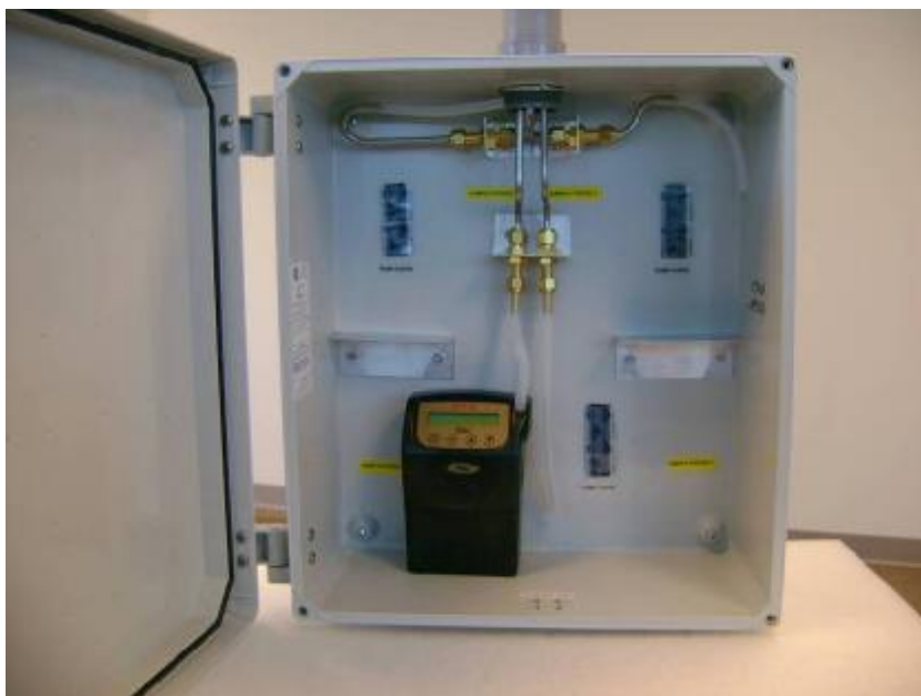
FIGURE 3. Diisocyanate Sampling System Enclosure
