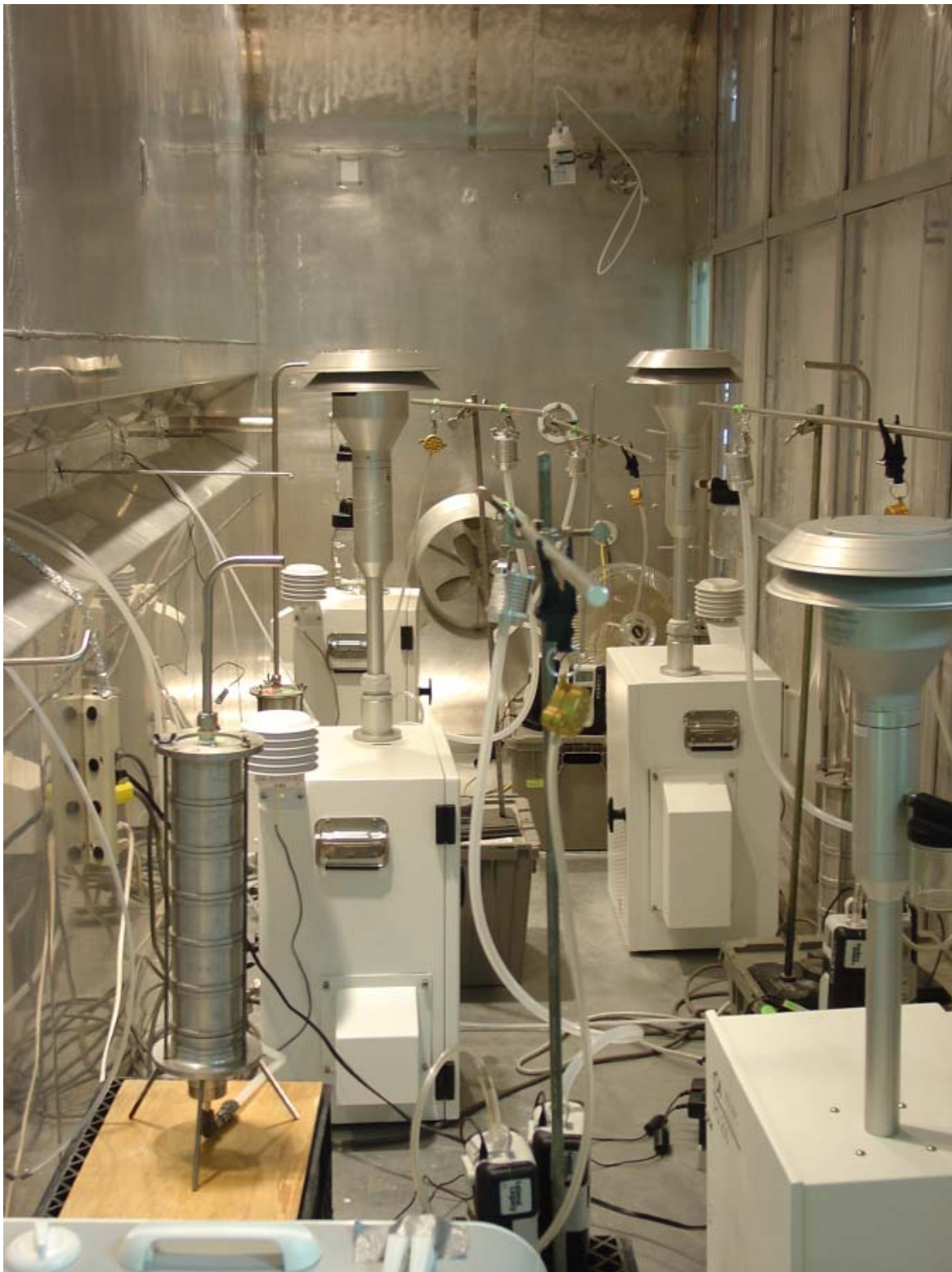
Figure 3-7. Test and Reference Particle Samplers Inside the Battelle Environmental Chamber Just Prior to Aerosol Generation for the Sampling Efficiency Testing.
