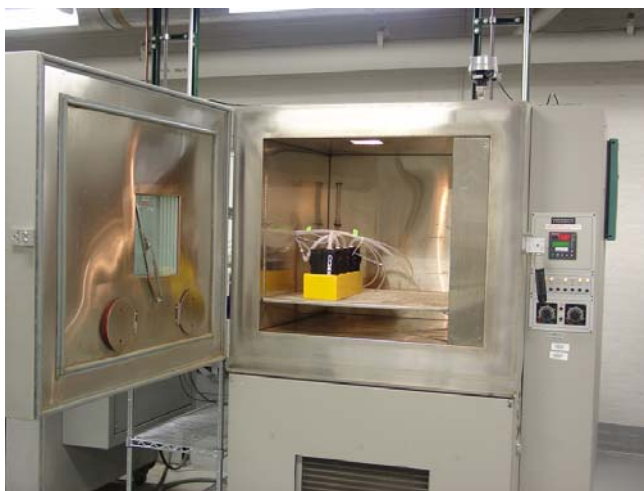
Figure 3-1. Leland Legacy ® Pumps (4) Inside the Constant Temperature and Humidity Chamber.
