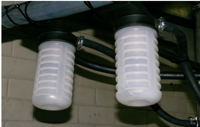
Figure 1-1. NCI Condensator on the Cummins N-14 Test Engine
