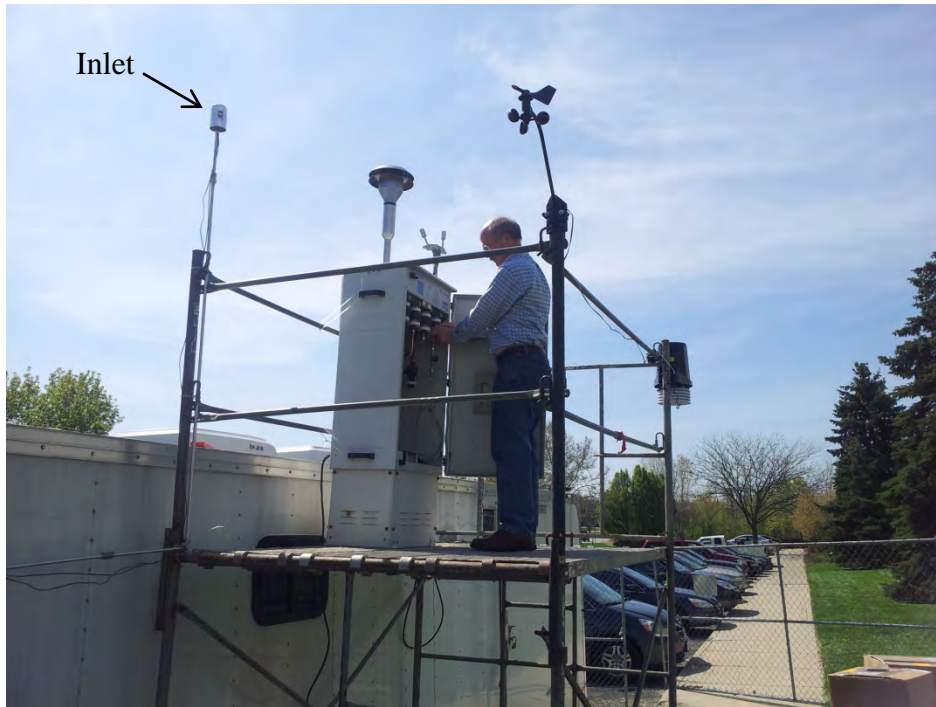
Figure 3-3. RAAS reference sampler installed at sampling site.
