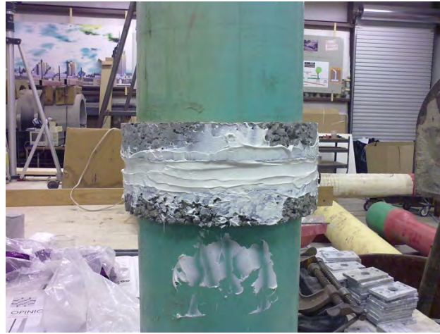
(b) Repaired cracked concrete with epoxy grout.
