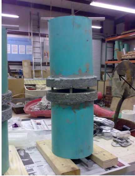
(a) Simulated cracked concrete.
