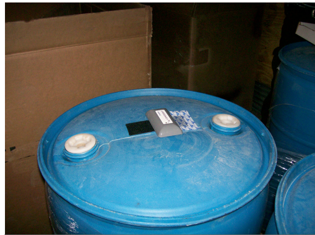
Figure 3-1. RFID tag affixed to poly drum
