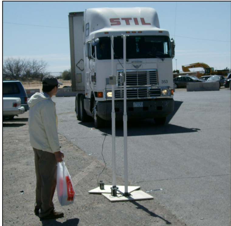
Figure 3-5. Stationary Tag Read with External Readers
