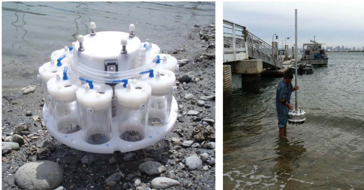
Figure 4. Second Generation SEA Ring Device (left). Field Evaluation in Beach Deployment (right)
