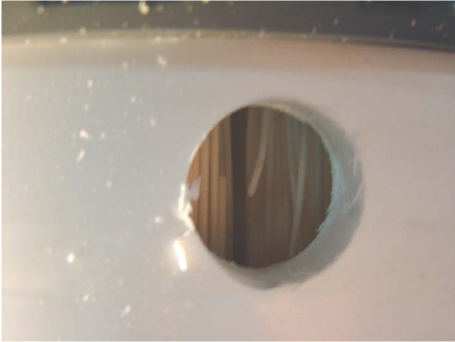
Figure 3-1. Photo of a cut fiber in one of the Dow SFD-2880 modules tested.
