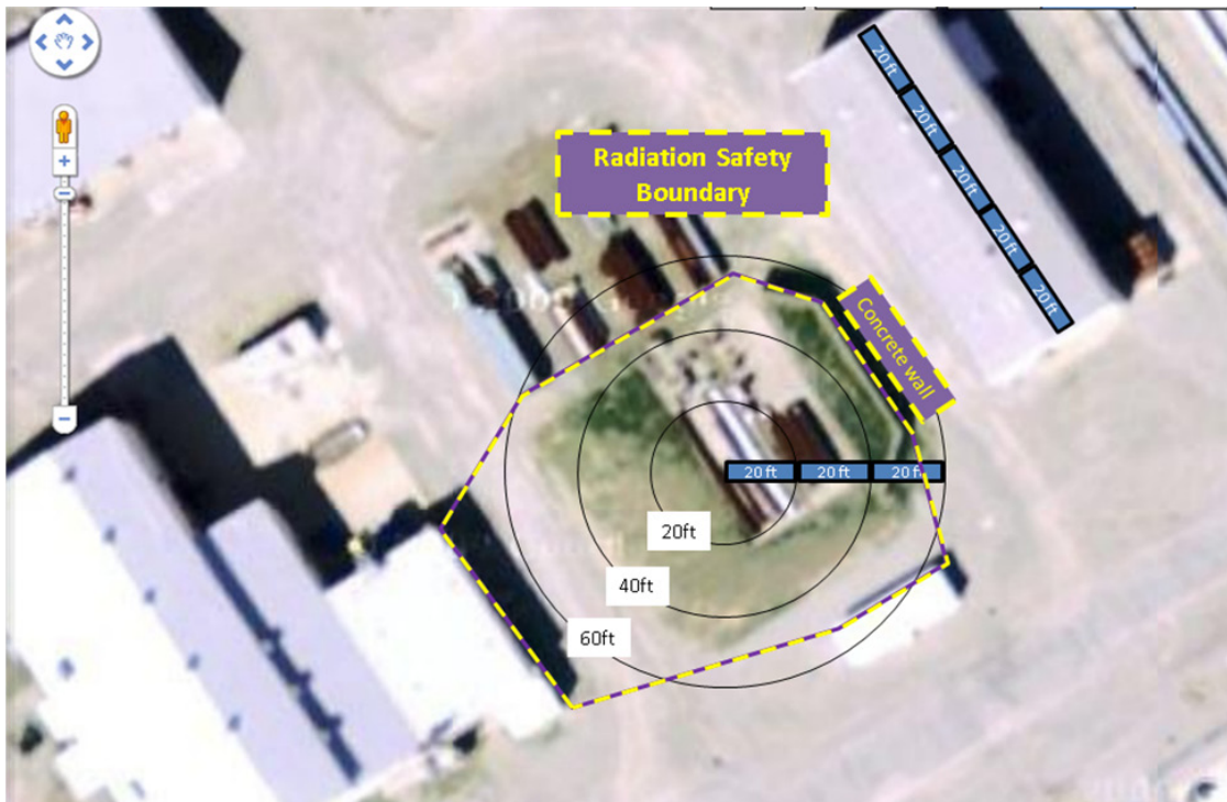
Figure 6-5. Radiation safety boundary for the operation of the VJ Technologies IXS High Frequency Integrated X-Ray Generator.
