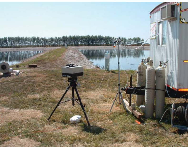
An Ambient Ammonia Monitor at an AFO
