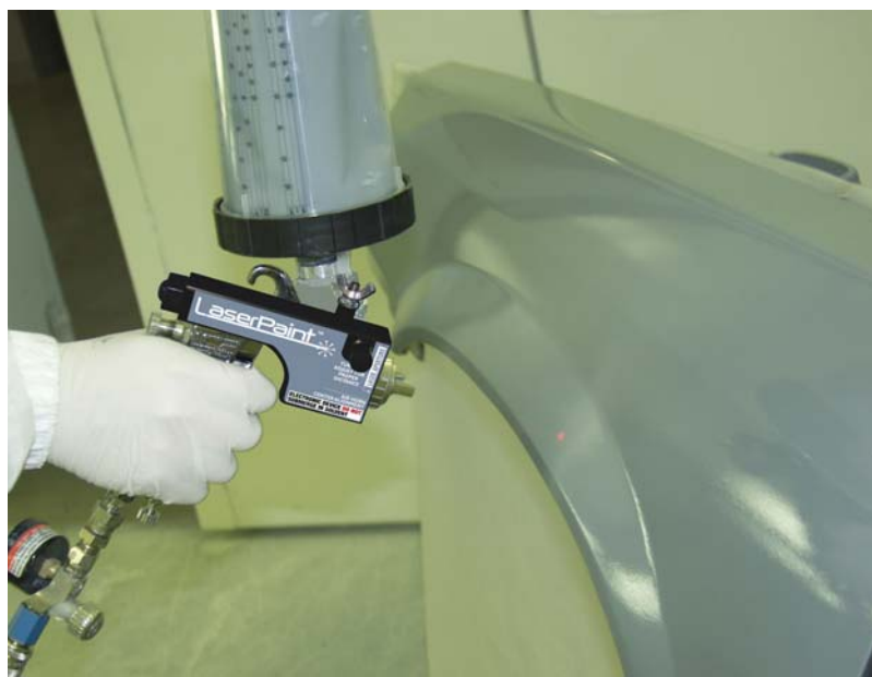
The laser targeting technology applied to a fender
