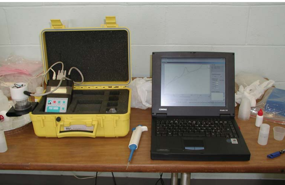
Two of the ETV-verified lead in dust analyzers (R. Jenkins, ORNL. Library of Lead in Dust Monitor Verification Photographs.)
