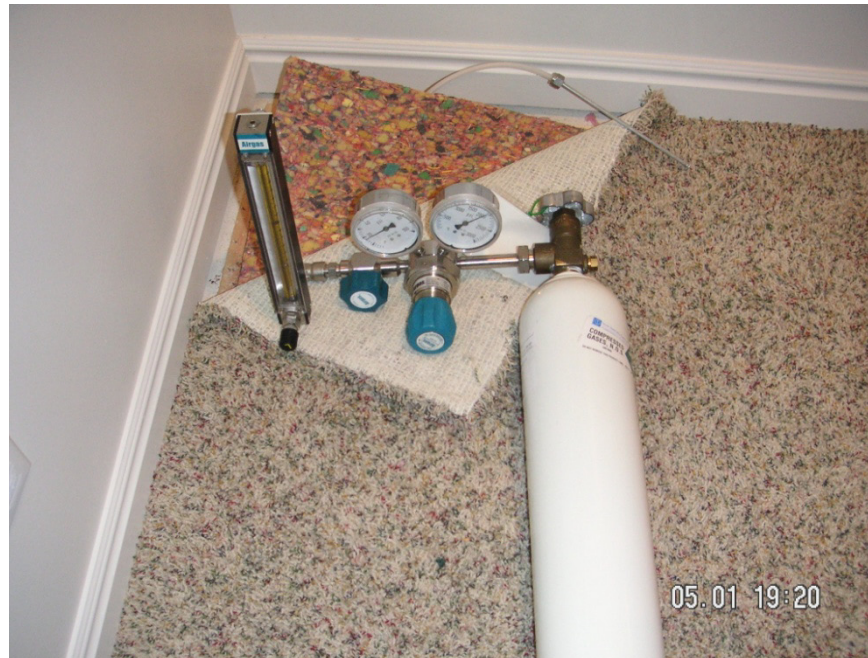
Figure 4. SF 6 Tracer Gas Delivery System for Determination of Building AER (Photo courtesy Dr. Thomas McHugh, GSI.)
