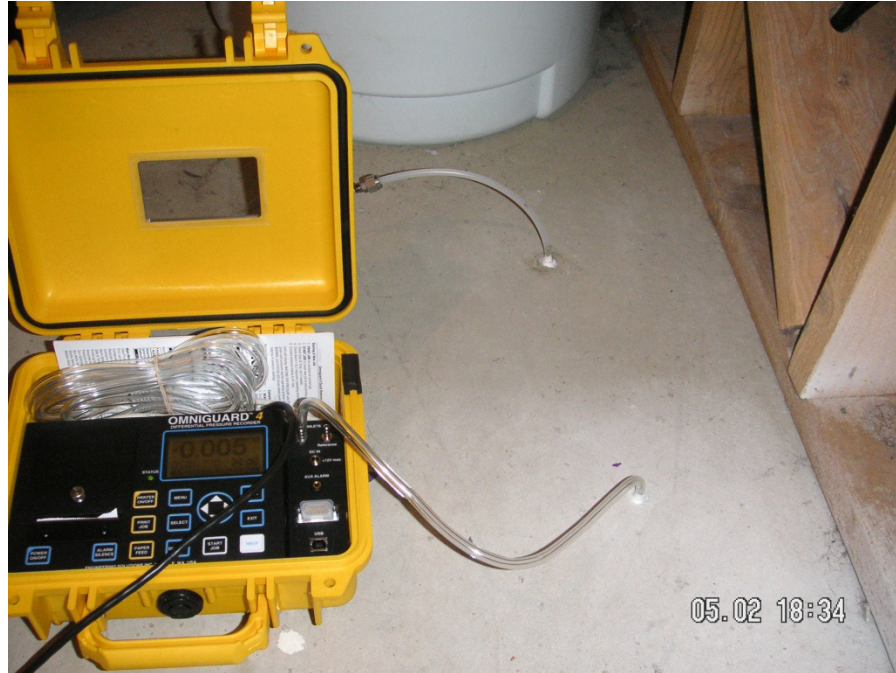
Figure 5. Real Time Pressure Transducer Installed to Measure Cross-Foundation Pressure Differential (Photo courtesy Dr. Thomas McHugh, GSI.)
