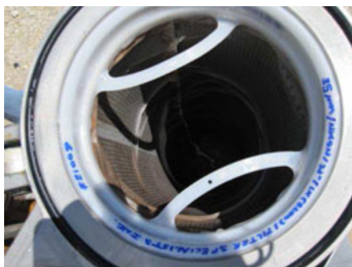
Figure 8. Nylon monofilament mesh filter bag secured in an Eaton Toplevel™ filter housing.
