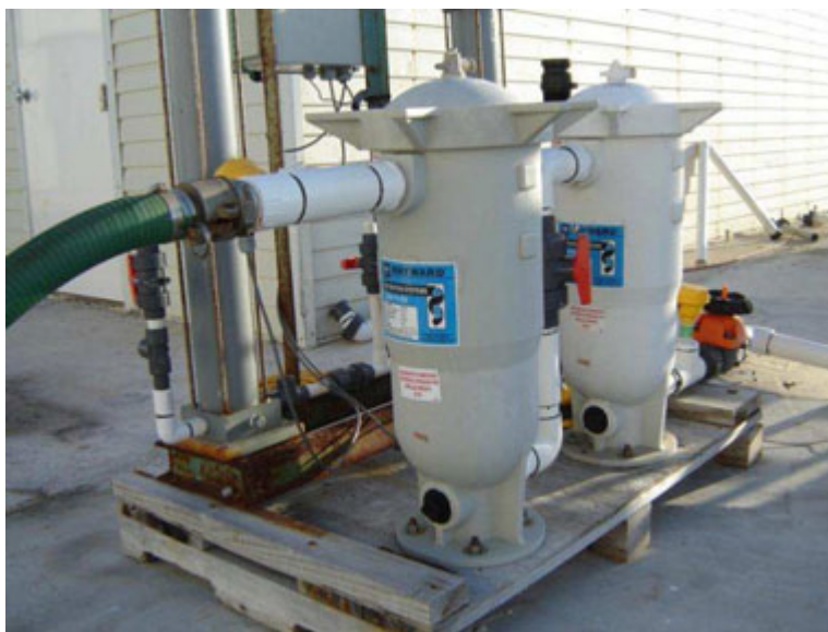
Figure 1. Two 41 cm long filter bags in Hayward housing arranged in series; water entered the system via the green hose at the top of the left-hand housing.
