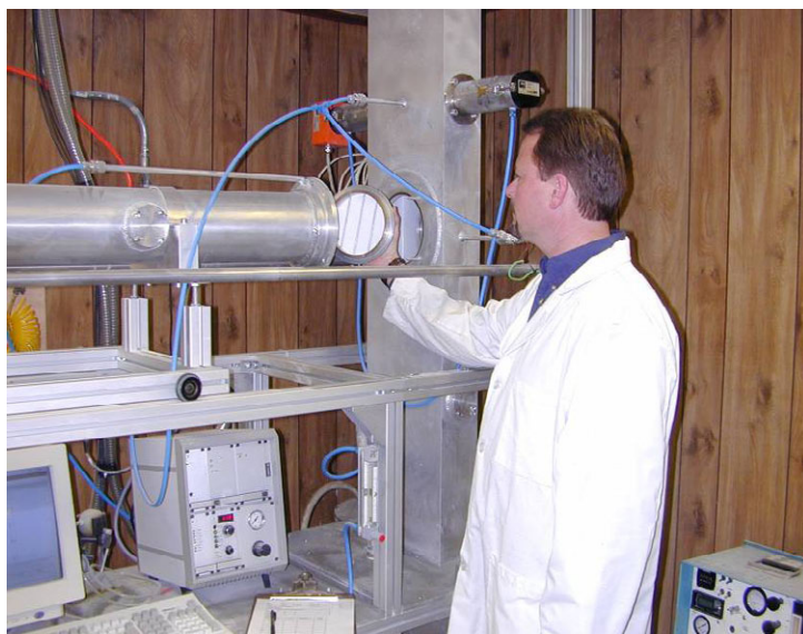
Installing a fabric swatch in the test apparatus at ETS Incorporated
