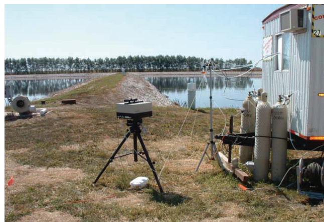
An Ambient Ammonia Monitor at an AFO
