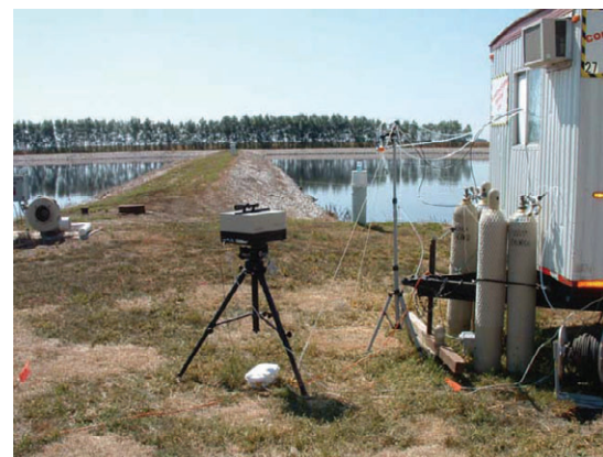
An ambient ammonia monitor at an AFO
