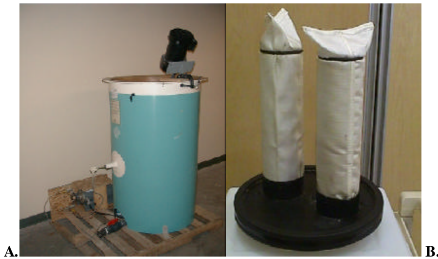
Figure 2-2. Components of Separmatic™ DE Pressure Type Filter System A. Body Feed Tank B. Filter Septa
