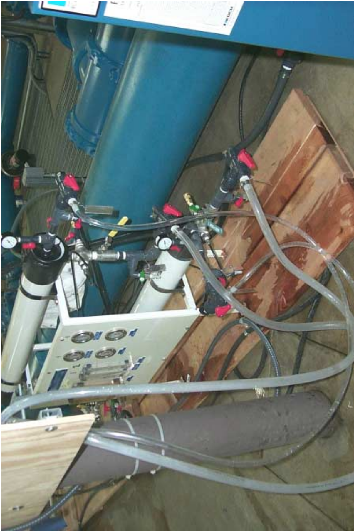
Photograph 4: Membrane Element Module Test Unit showing permeate and concentrate end of module
