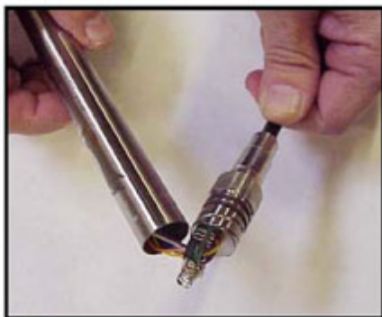
Figure 4a: Gently separate the top-cap from the body of the sensor. Top-cap remains attached to body via several colored wires.
