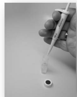
Transferring Spike Solution to Sample Tube
