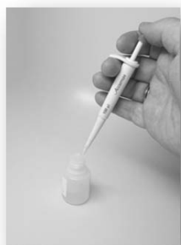
Withdrawing Standard Solution Using Pipette
