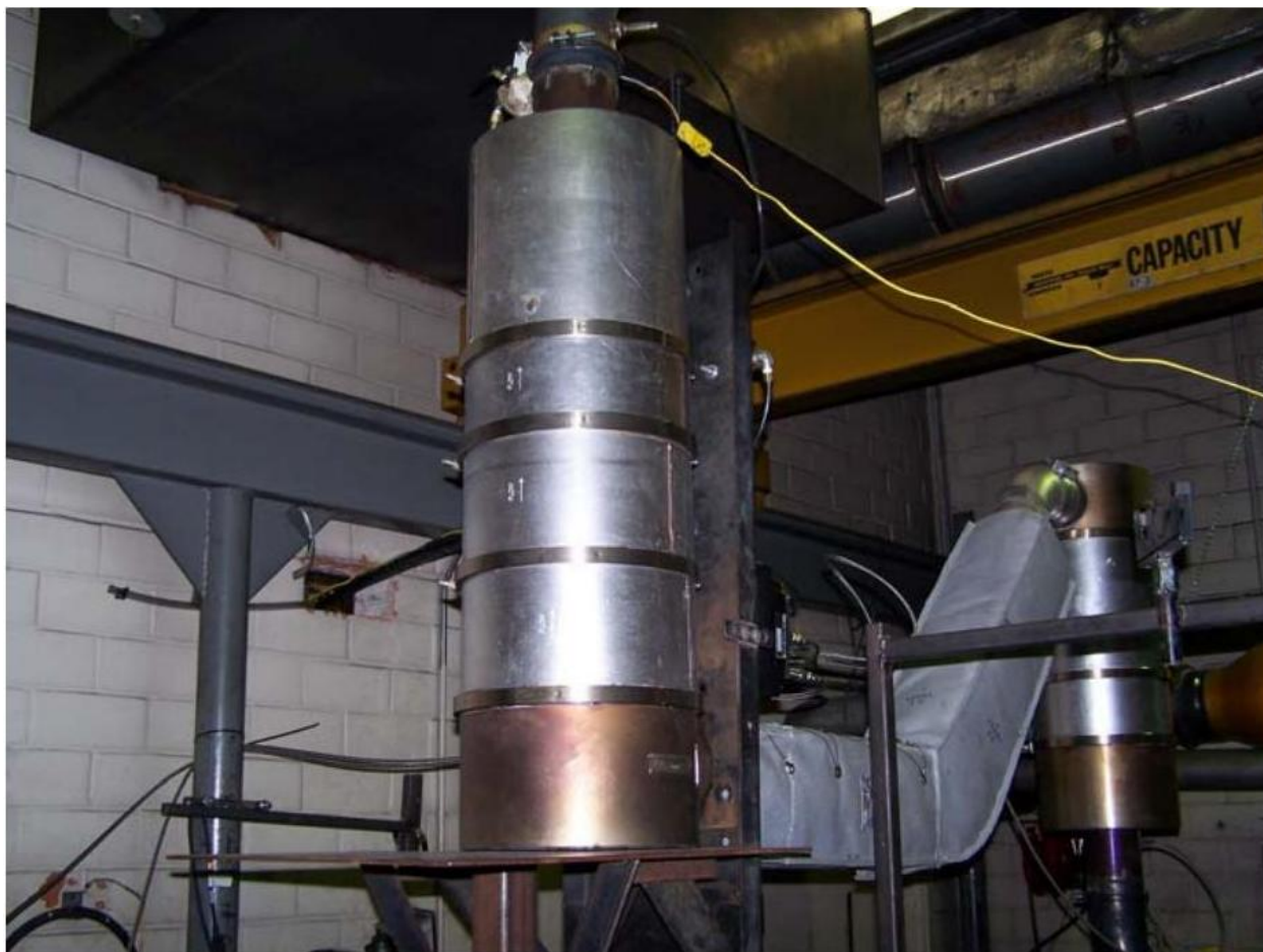
Figure 3. The degreased SCCRT ® , v.1 system installed for emissions tests in February 2011.
