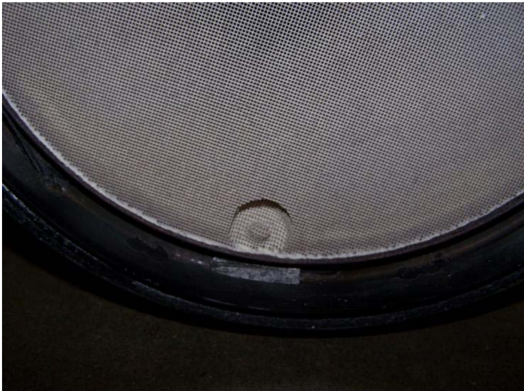
Figure 7. Photograph of the aged CRT catalyst erosion caused by the loose fastener.
