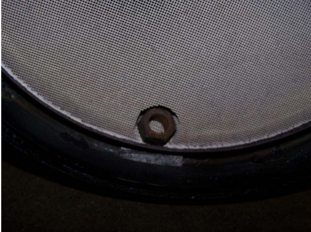
Figure 6. Photograph of the loose fastener found in the aged CRT catalyst after the March 2010 emissions tests.
