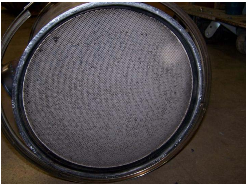
Figure 8. Photograph of the aged CRT filter face.
