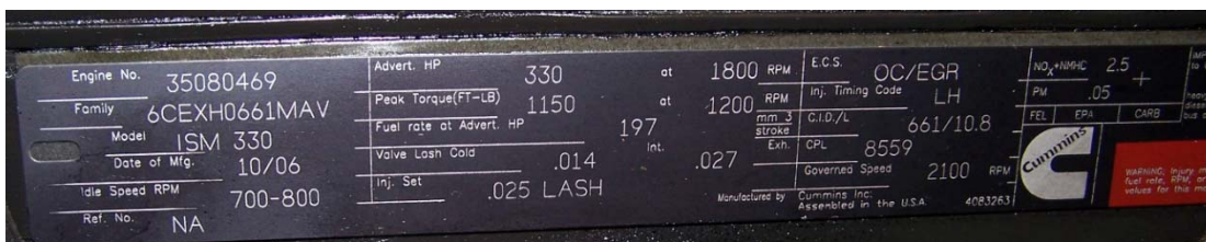
Figure 4. Identification label for 2006 Cummins ISM 330 engine.
