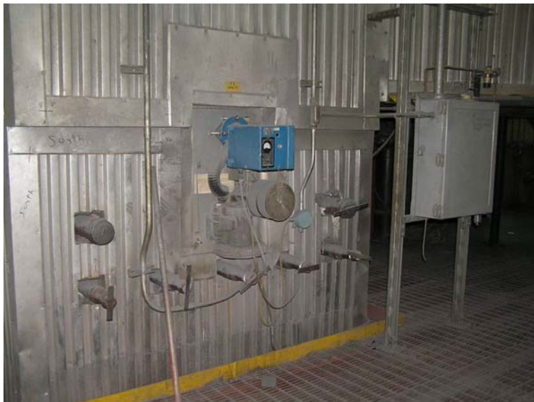
Figure 2-2. Emission Testing Ports for MP-5
