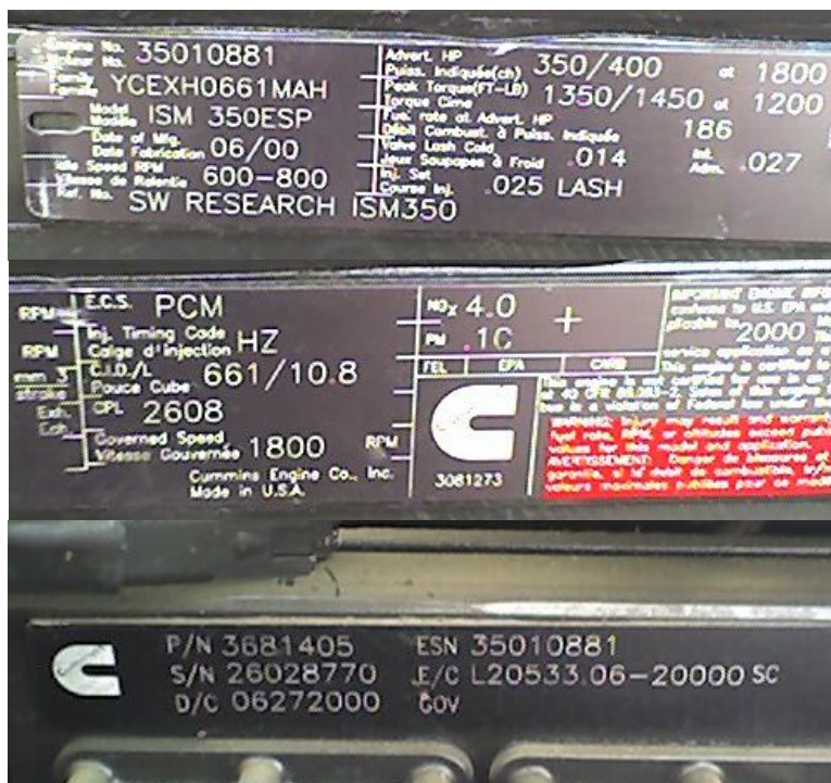
Figure 3. Identification labels for 2000 Cummins ISM350 engine and its electronic control module.
