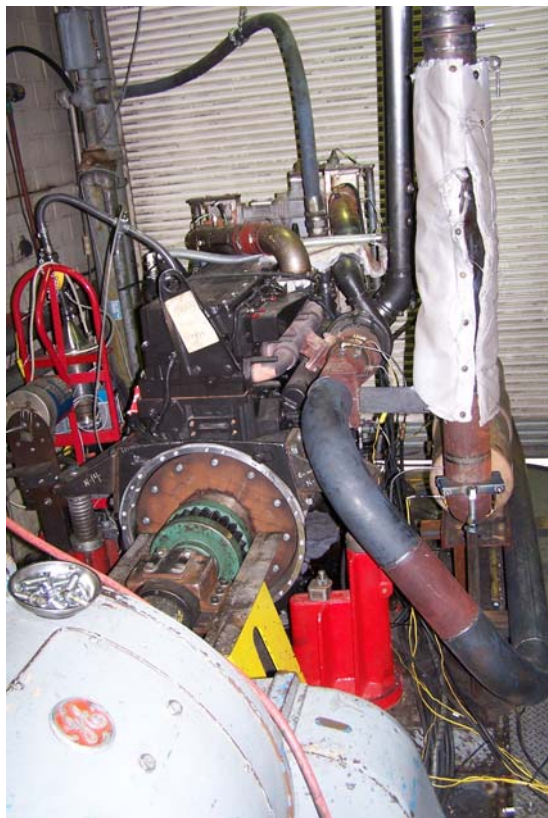
Figure 1. Engine shown in emissions test cell with Cummins DOC+CCV installed on engine.
