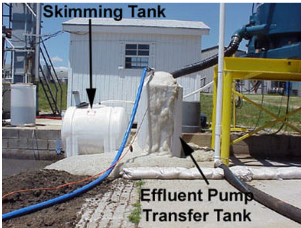
Figure 4-1. Foam produced with the TS-5000 effluent.
