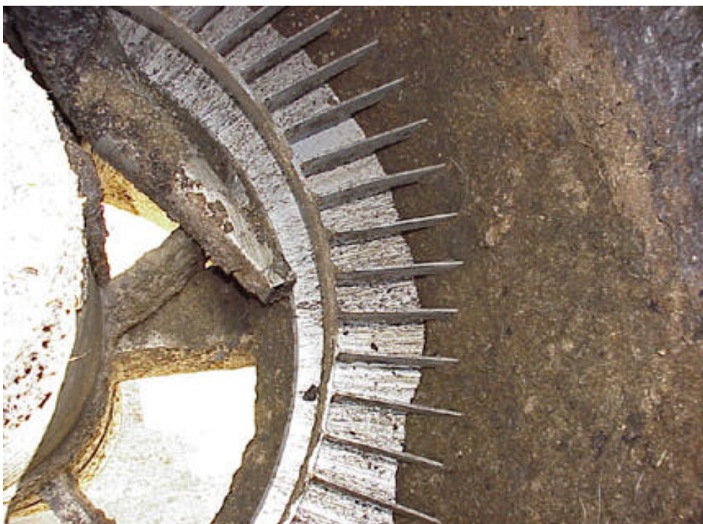
Figure 3-3. Internal view of TS-5000 showing feed tube at the bottom of the bowl.
