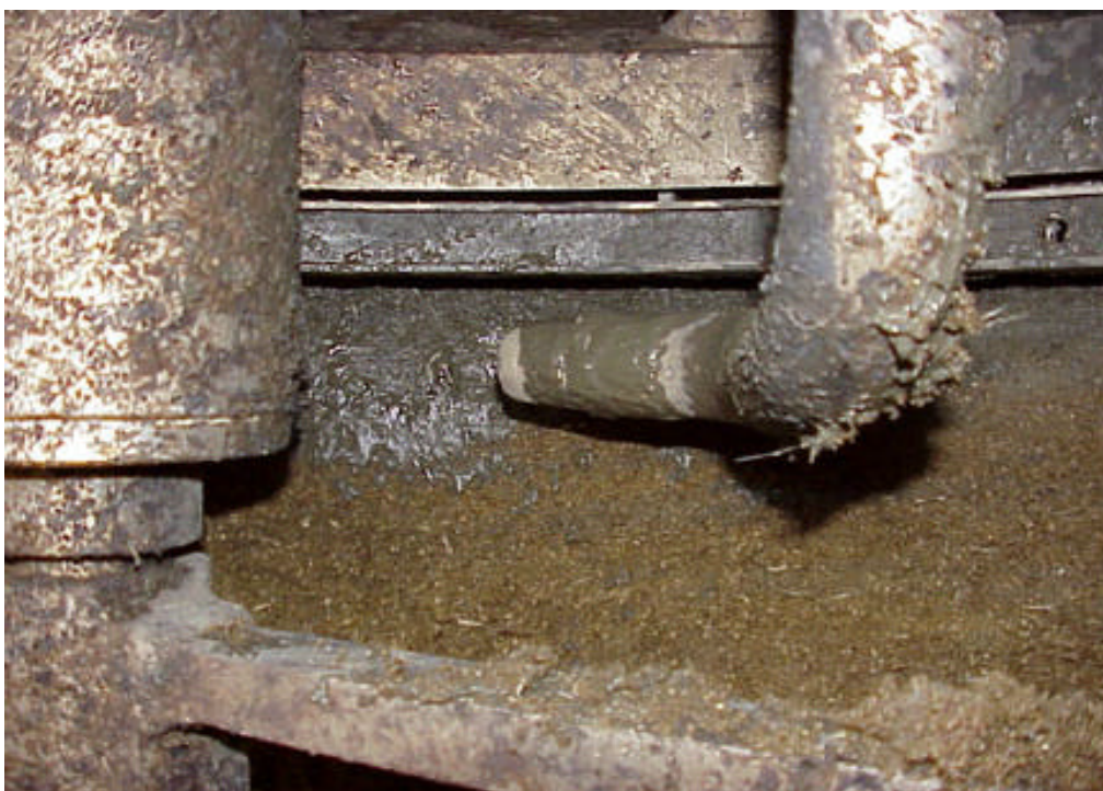
Figure 3-5. Internal view of TS-5000 showing the skimming tube at the top of the bowl.
