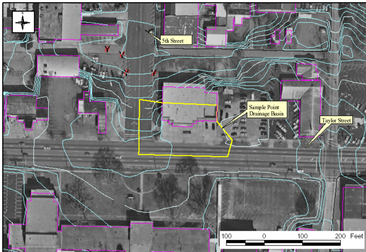
Figure 3-2. Drainage basin map for the StormFilter installation.
