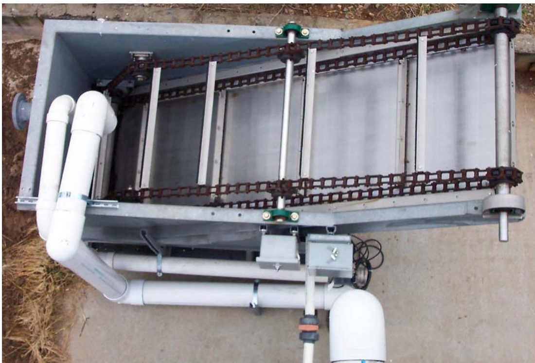
Figure 2-2. Hoffland Environmental Inc. inclined screen.
