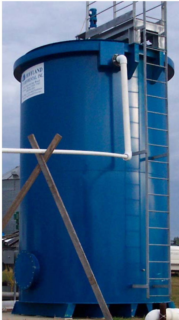
Figure 2-1. Hoffland Environmental Inc. clarifier.
