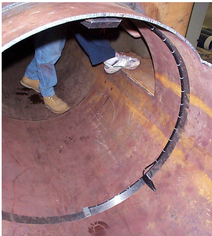
Figure 3-9. ADS flow monitoring sensors (laboratory 42-inch pipe installation).
