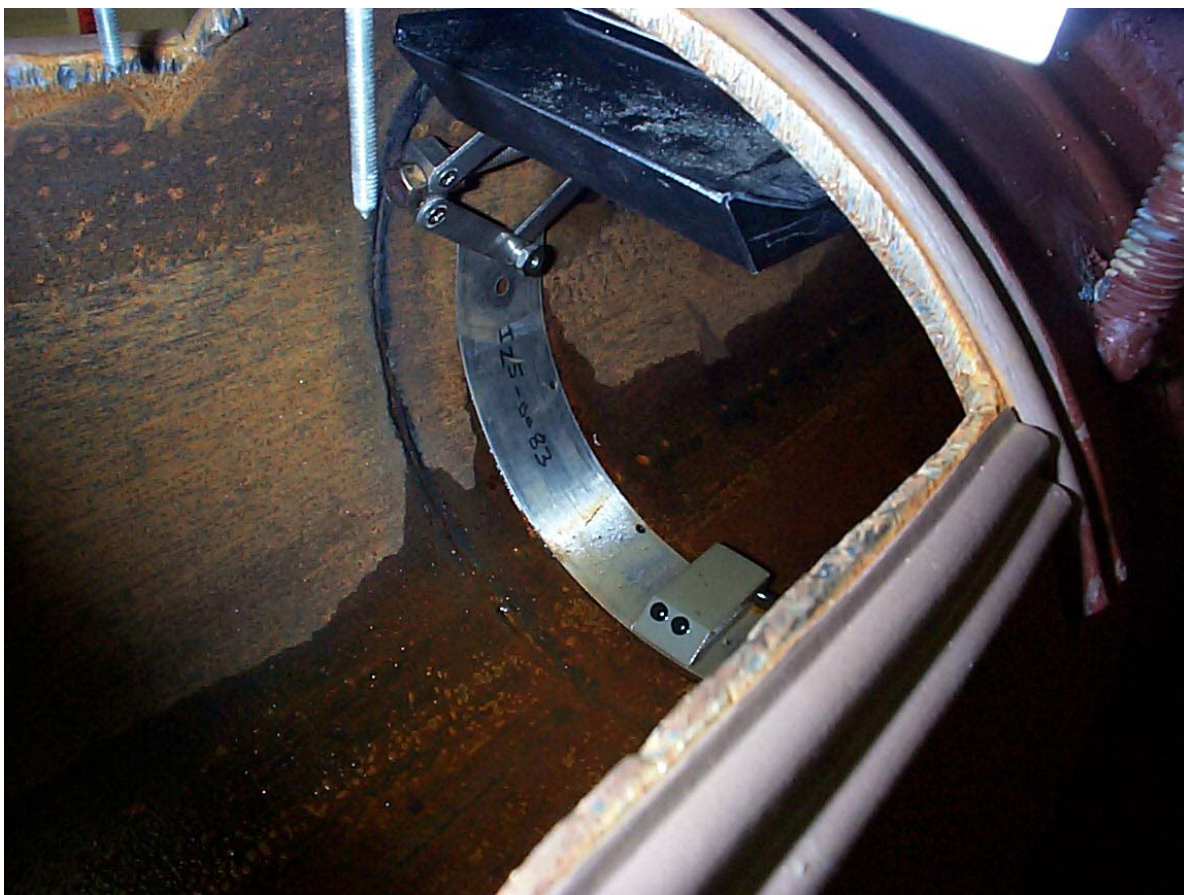
Figure 3-8. ADS flow monitoring sensors (laboratory 10-inch pipe installation).
