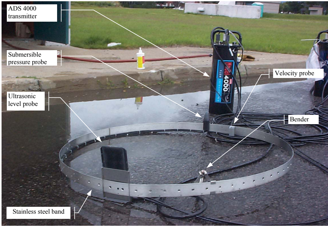
Figure 4-10. ADS 4000 flow meter components.
