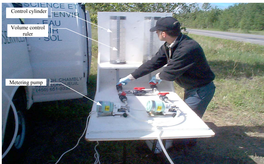
(a) Lithium injection control system.
