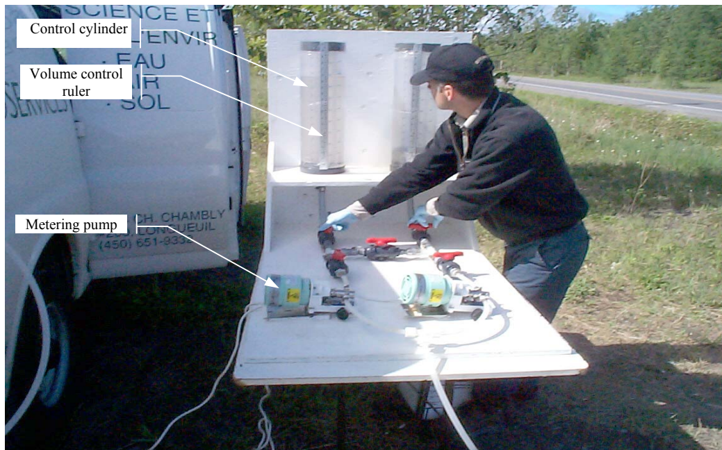
(a) Lithium injection control system.
