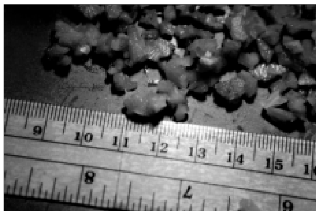
Figure 3-4. Intermediate Ammonium-Zinc Crystals
