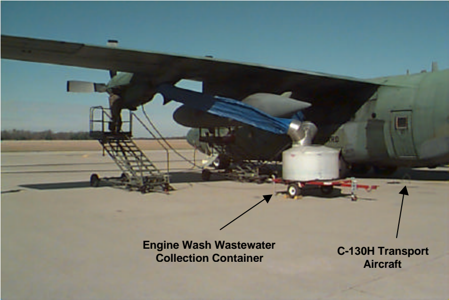
Figure 3. The 179 th AW Wash Wastewater Collection Container
