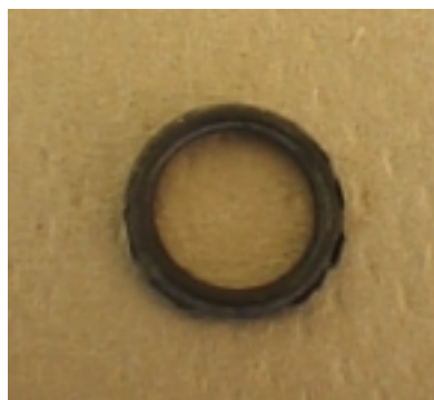
Figure 5 Inner O-ring Showing Wear
