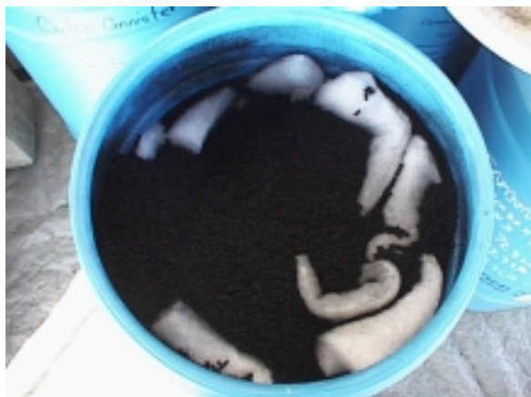
Figure 7 Carbon Filter with Upper Fiber Layer Removed
