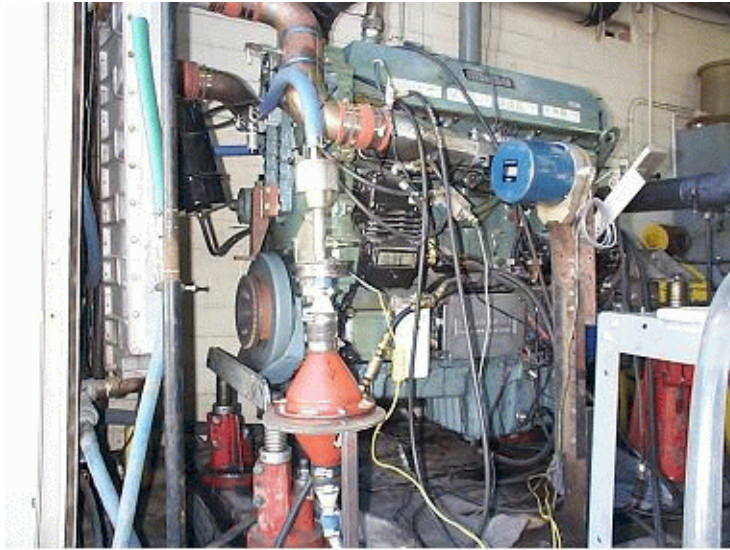
Figure 2. Baseline engine: a 1998 Detroit Diesel Corporation heavy-duty diesel engine, mounted in Southwest Research Institute's engine test cell #4.
