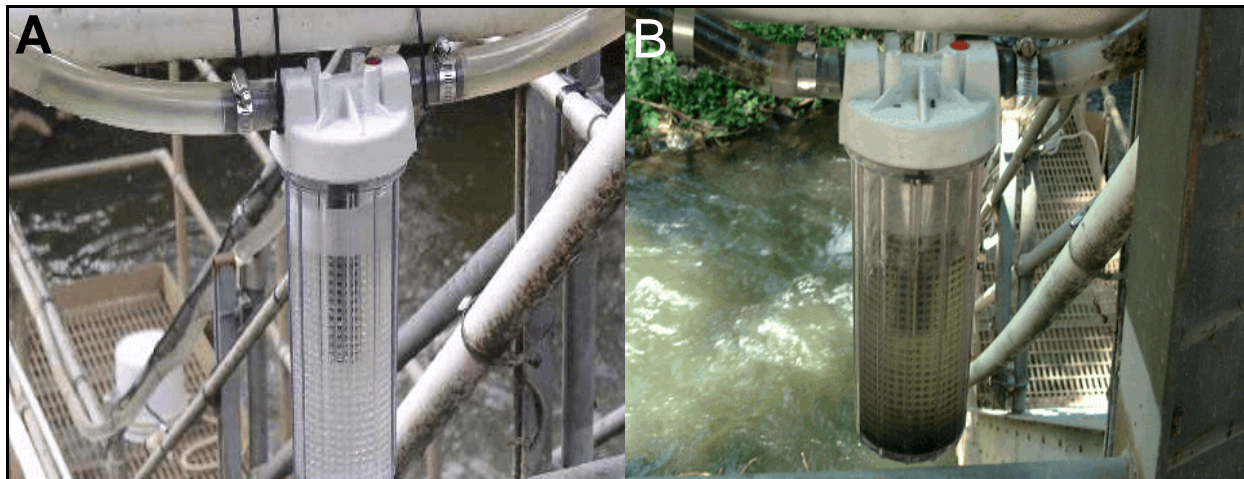
Figure 3-4. In-line Filter Screen and Inlet Tubing Before (A) and After (B) the Verification Test
