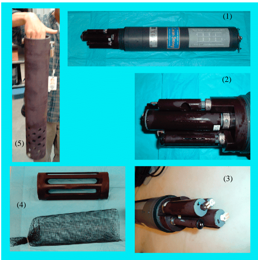
Figure 6-1. 6600 EDS Prior to Deployment. Starting in the upper right and proceeding clockwise: (1) clean 6600 EDS, (2) close-up of clean probes, (3) close-up of wiping brushes, (4) protective shroud and mesh, (5) aluminum tube guarding against crushing damage.
