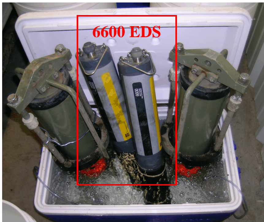
Figure 6-3. Cleaned and Reconditioned 6600 EDSs in Storage Tank Used Between Deployments
