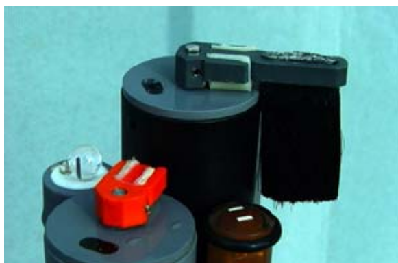
Figure 2-1. YSI 6600 EDS Water Probe
