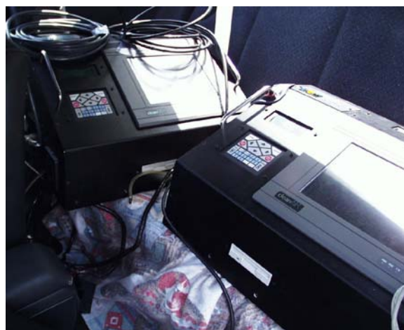
Figure 3-3. View of the Duplicate REMOTE OEMs in the Chevy Tahoe Before On-Road Testing
