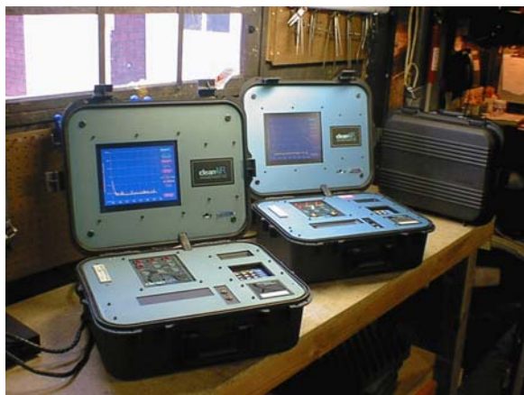
Figure 2-1. Clean Air Technologies REMOTE On-Board Emissions Monitor
