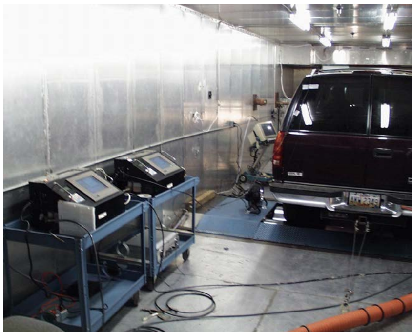
Figure 3-1. Chevy Tahoe in Dynamometer Cell
