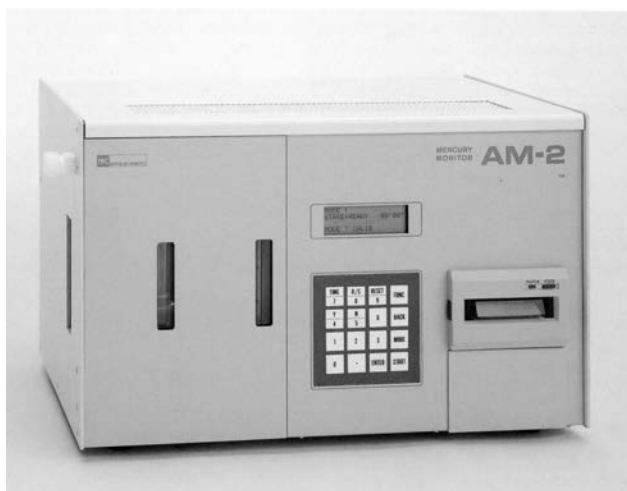
Figure 2-1. Nippon Instruments Corporation Model AM-2 Mercury Continuous Emission Monitor
