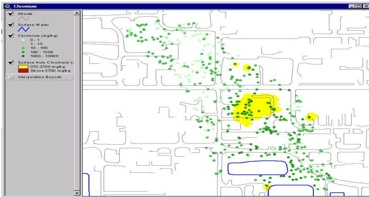
Figure 6. ArcView with Spatial Analyst chromium contamination map at 370 and 3700 mg/kg thresholds.
